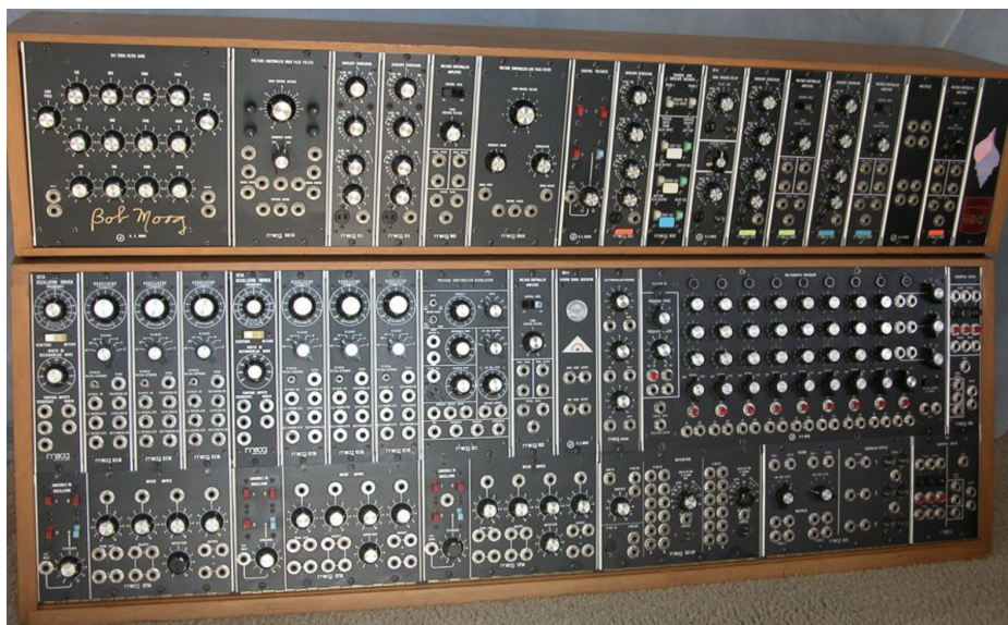
Figure 5: One of Moog’s modular synthesizers. The inputs and outputs used for patch cords can be seen all throughout the surface of the instrument.[2]
