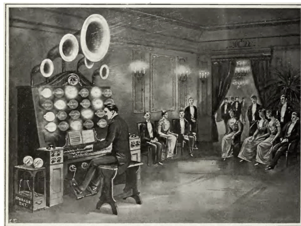
Figure 2: A sketch of the Audion Piano in action. Due to the components available at the time, the instrument needed to take up a large amount of space.[6]
