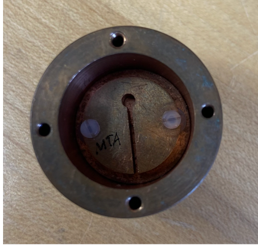
Figure 12: A prior monomodal Loop Gap Resonator shown sitting on washers inside of copper shield.
