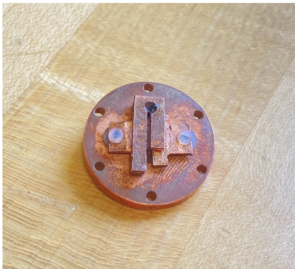
Figure 20: New bimodal resonator shown on copper shield cap. Resonant Frequencies are variable with bending of prongs. Generally around 4 and 5.3 GHz.
