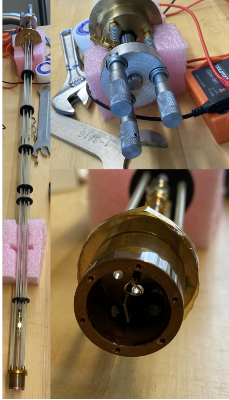
Figure 14: Adjustable sample probe. Shown with entire apparatus (left), shield with inductive loop inside (bottom right), and micrometer adjustments (top right).
