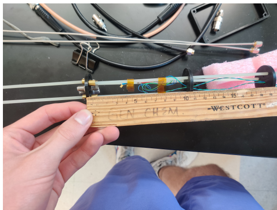
Figure 4.7: The placement of the movable thermistor in the second baffle region, with a ruler as a fiducial.
