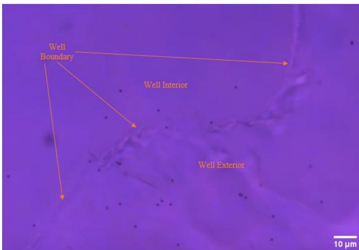
Figure 4. Bright-field microscope image of a 1.75 mm tall agarose hydrogel well boundary using 20x magnification.
