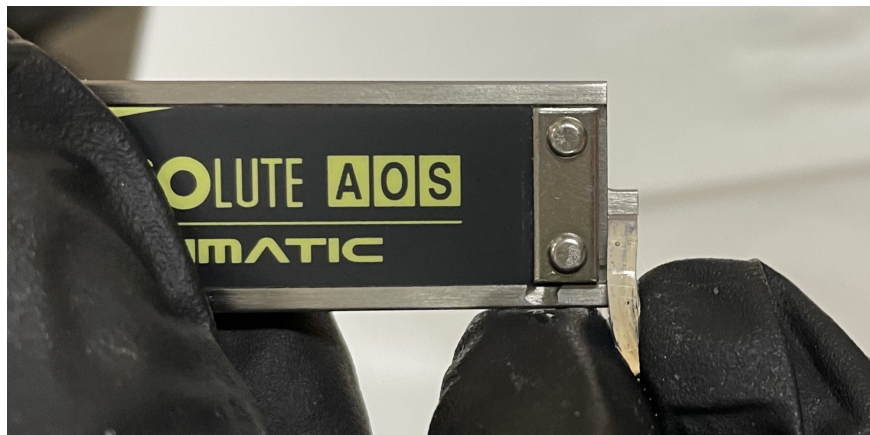
Figure 10: Image of the developed measuring technique using calipers which allows for the measurement of soft agarose gel without distortion of the cylinder.
